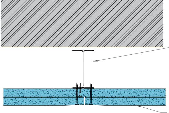
· SPEEDLINE 70mm 'I' Studs at 600mm Ctrs
